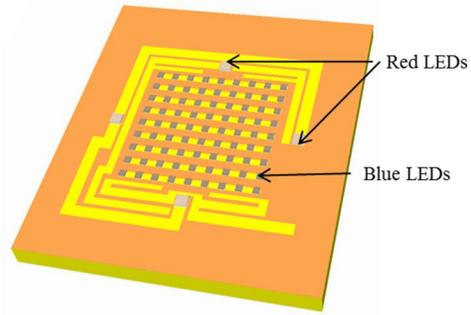
Fig. 5. LED module layout in the thermal simulations.
