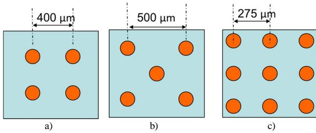
Fig. 4. (a) 4 via configuration (b) 5 via configuration (c) 9 via configuration tested under the blue LED chips on Cu MCPCB module.
