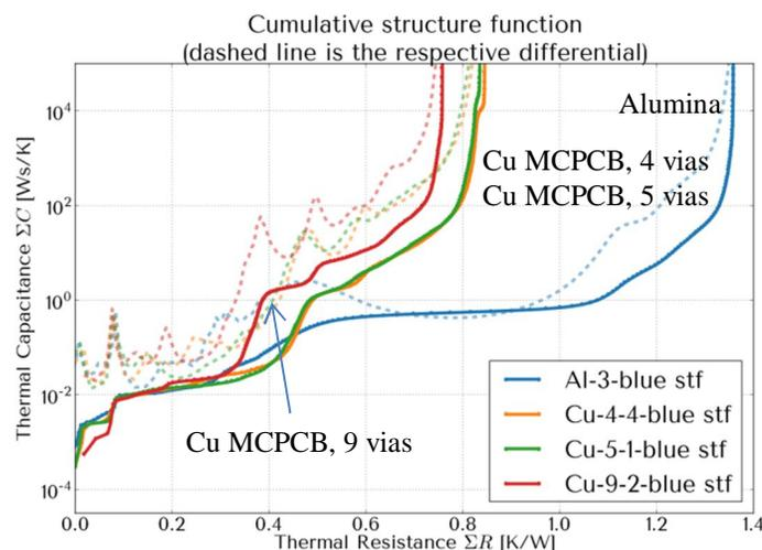
Fig. 9. Structure function of blue chip array on alumina module (blue) and on Cu MCPCB module with 9 vias (red), 5 vias (green) and 4 vias (orange) per chip.
