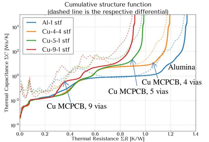
Fig. 8. Structure function of alumina module (blue) and Cu MCPCB module with 9 vias (red), 5 vias (green) and 4 vias (orange) under a blue LED chip. Dashed lines are differential structure functions.
