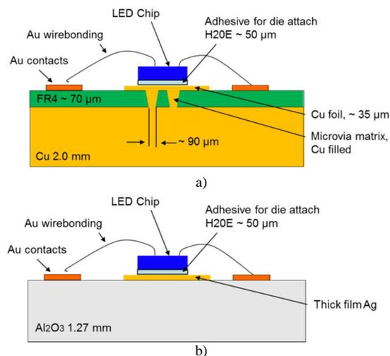
Fig. 3. (a) Cu MCPCB and (b) alumina test structure with blue LEDs.
