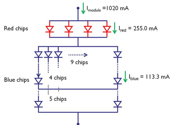
Fig. 1. Simplified electrical circuit of the LED module.
