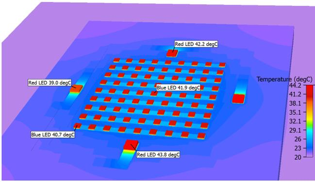
Fig. 6. Simulated surface temperatures on COB Cu MCPCB module with 4 microvias under each blue LED.
