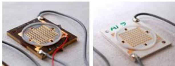
Fig. 2. Cu MCPCB module (left) and alumina module (right).
