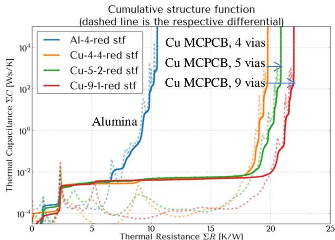
Fig. 10. Structure function of red chip array on alumina module (blue) and Cu MCPCB module with 9 vias (red), 5 vias (green) and 4 vias (orange).
