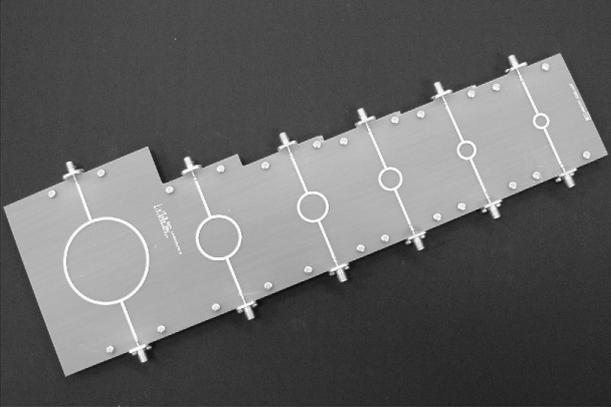
Fig. 1. The Measurement structure, which includes 1, 2, 3, 4, 5 and 6 GHz microstrip ring resonator.
