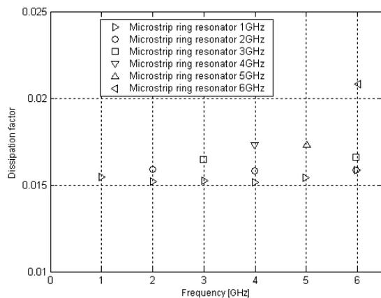
Fig. 4. The average values of the dissipation factor. (FR-4 RC ~40,3%)
