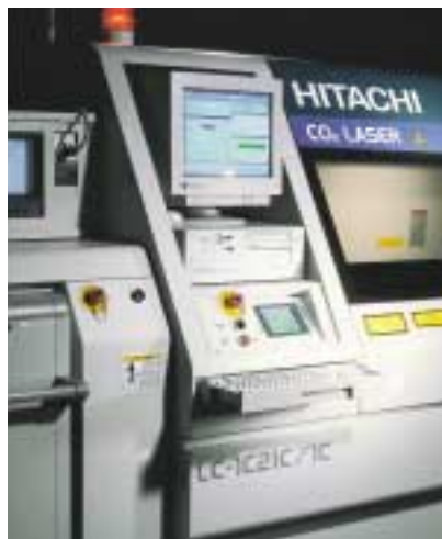
Laser drilling machine for HDI products.
